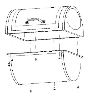
Connect firebox and grill base (item #9) together using six M6 x 15mm Phillips head bolts.
